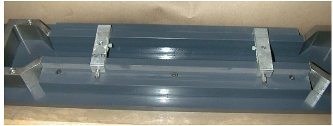
Figure 3. Picture of the CLS Mold before the Placement of the Concrete
