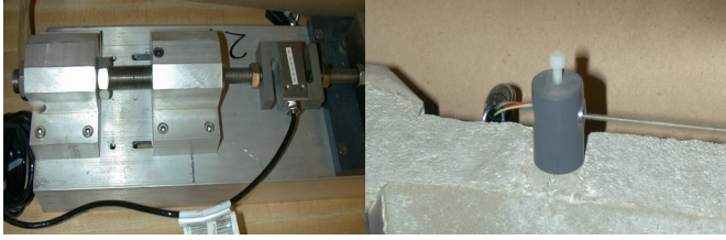
Figure 2. Picture of the Load cell and LVDT with holder in the CLS test set-up
